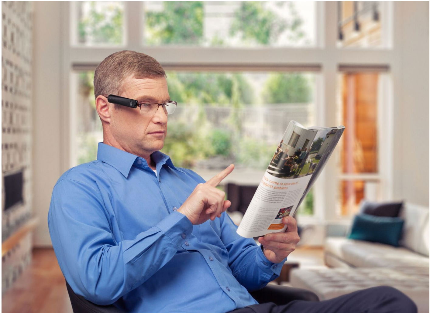
OrCam’s MyEye is an assistive device for the blind and visually impaired. It uses AI to read text, recognize faces and even identify products, transforming the lives of the visually impaired. © OrCam
